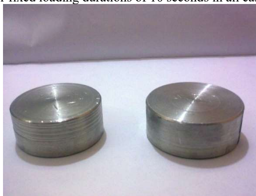
Fig. 4.9. Specimen employed for hardness test
